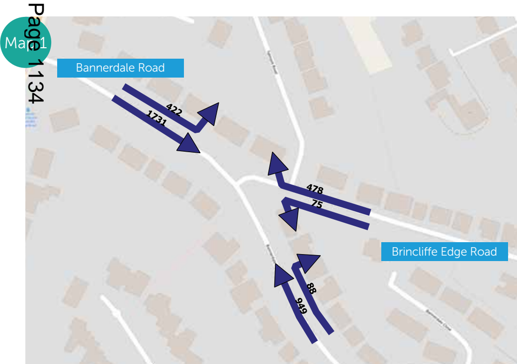
2 day average number of motor vehicles travelling through the Bannerdale Road / Brincliffe Edge Road junction before the scheme (May 2022)
